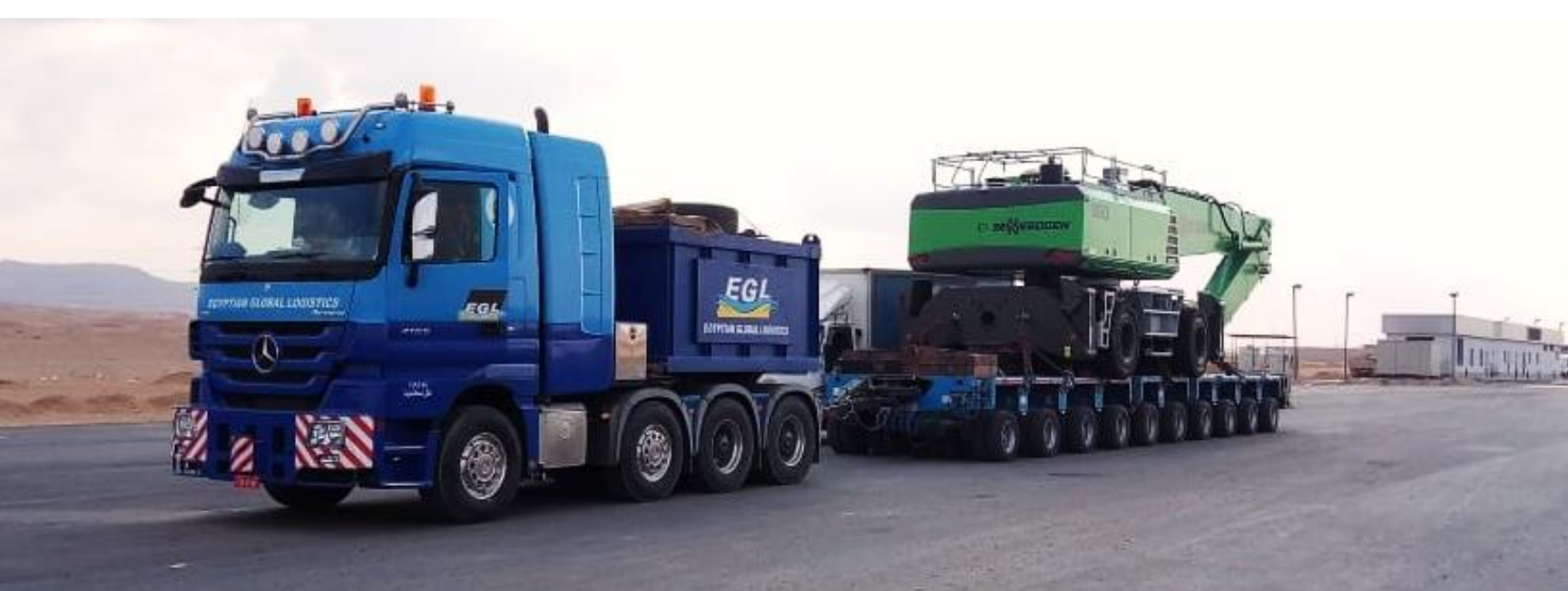
Transportation of Material Handler of 75 tons & 15.5 m long From Alex Port To Suez.
