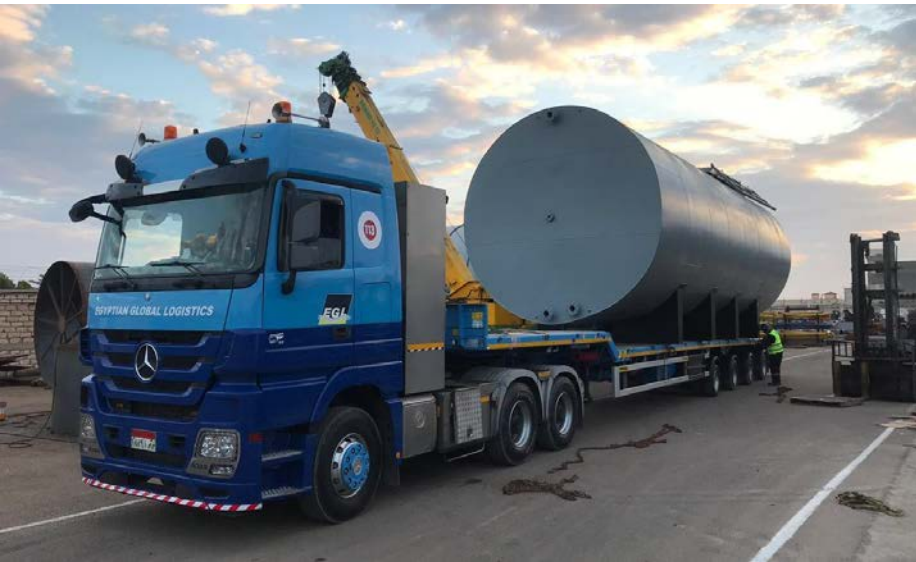
Transportation of tank 12m length & 4.6m diameter from Borg Al_Arab to Wahat 25 tons weight
