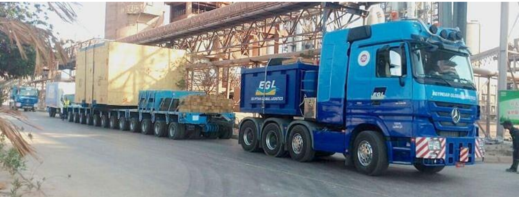
Discharging and Trucking of a 141 tons Gearbox unit from Alexandria port to El Arish Sinai.
