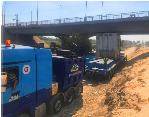
Trucking, discharging and storage of 4 *228 Ton and 2*60 Ton of Cairo west power plant project
