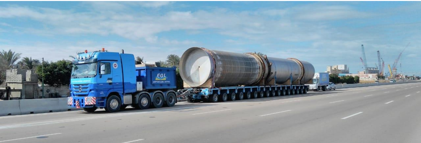
Loading & Transportation of a Fibre-flow of 71 tons, 24 meter length From Alexandria Port to paper factory In Cairo
