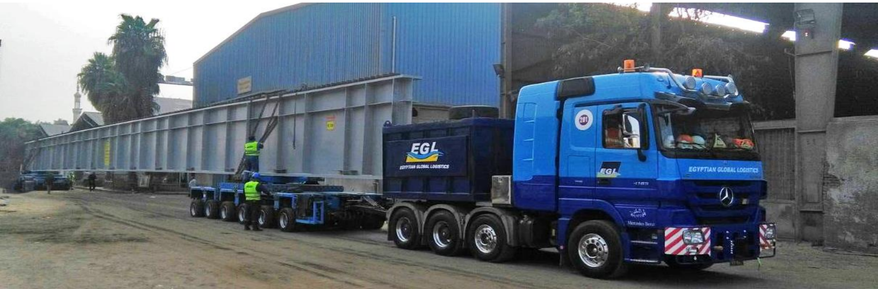
Trucking of 105 tons, 61 m long beams for Shobra El mazalat bridge Cairo using our special turn tables.
