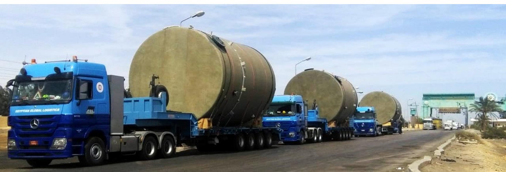
Discharging, Loading & Trucking of 4 over size tanks 8 m diameter each.
