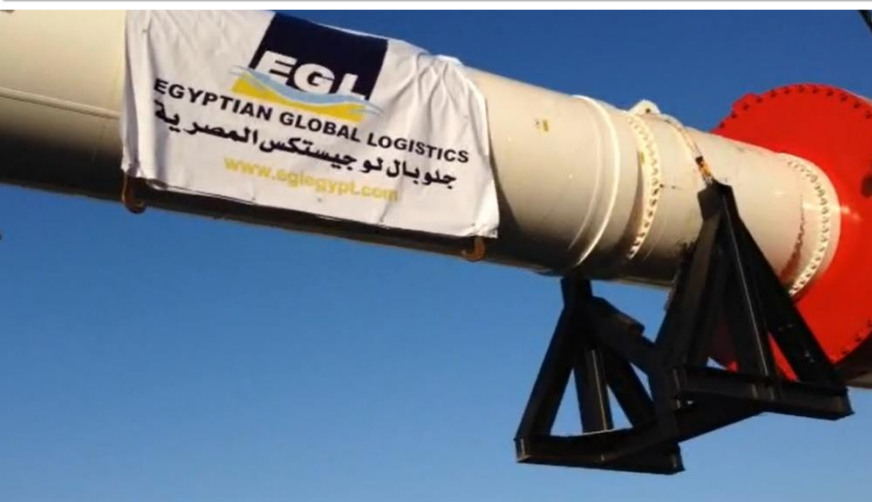
Discharging, Storage & Trucking of a 135-Tons Hammer, 22 m long from Port Said west to Port Said east new jetty.
