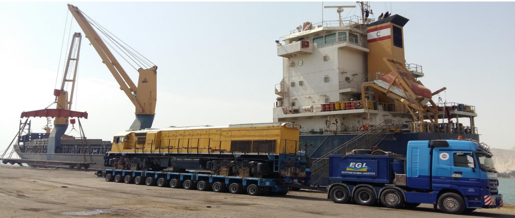
Discharging & trucking of 2 locomotive 3000 HP, 120 tons each at Adabyia Port to Orascom site at Abo Rawash “New Rail way project in Cairo”
