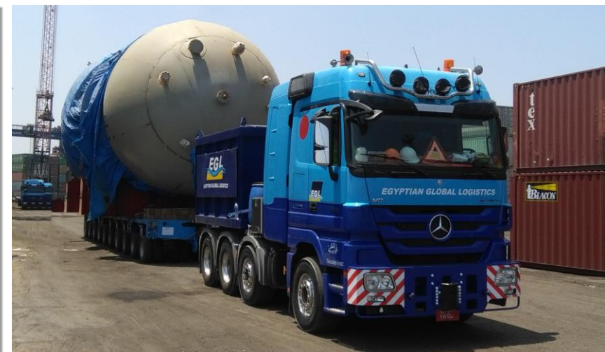
Trucking of Blow Down vessel unit of 72 tons, 17m Long & 6.4 Height from Alexandria to Sokhna
