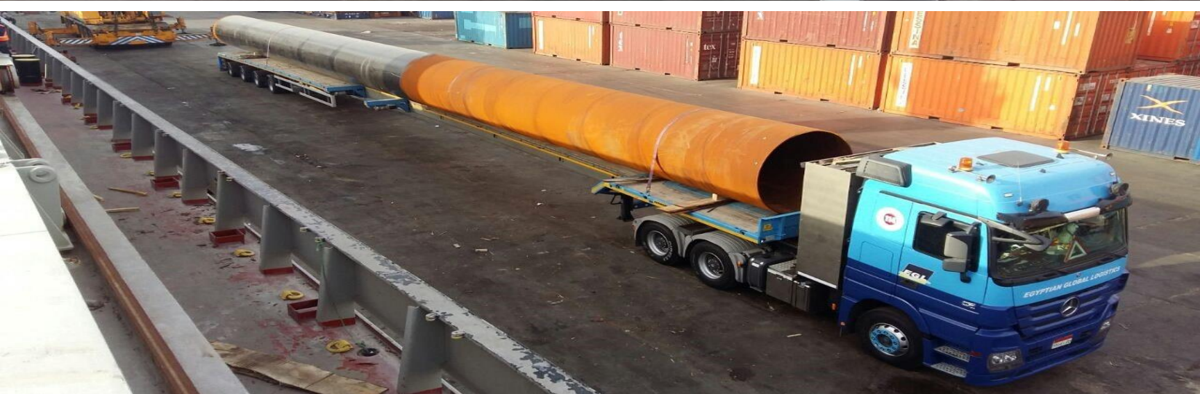
Trucking of pipes of 36 tons & 36 m long each at Alexandria port.
