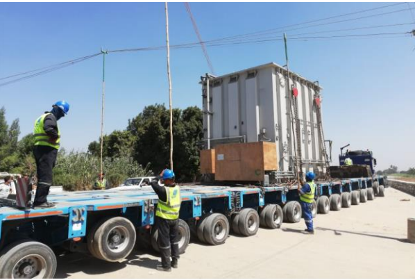
Trucking, discharging and storage of 4 *228 Ton and 2*60 Ton of Cairo west power plant project
