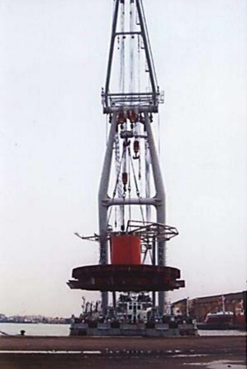
Loading a 230-ton, 17 m in diameter Egypt Internet Turntable
