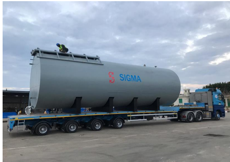
Transportation of tank 12m length & 4.6m diameter from Borg Al_Arab to Wahat 25 tons weight
