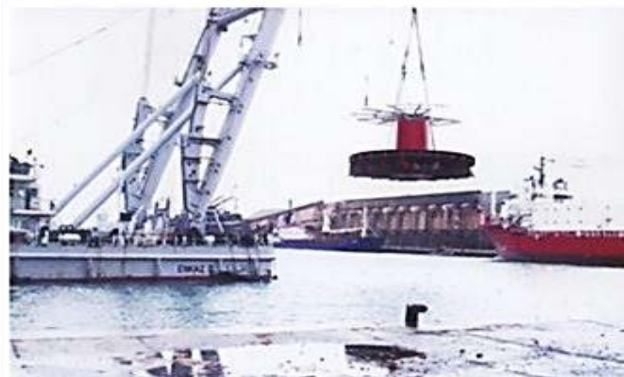
Loading a 230-ton, 17 m in diameter Egypt Internet Turntable
