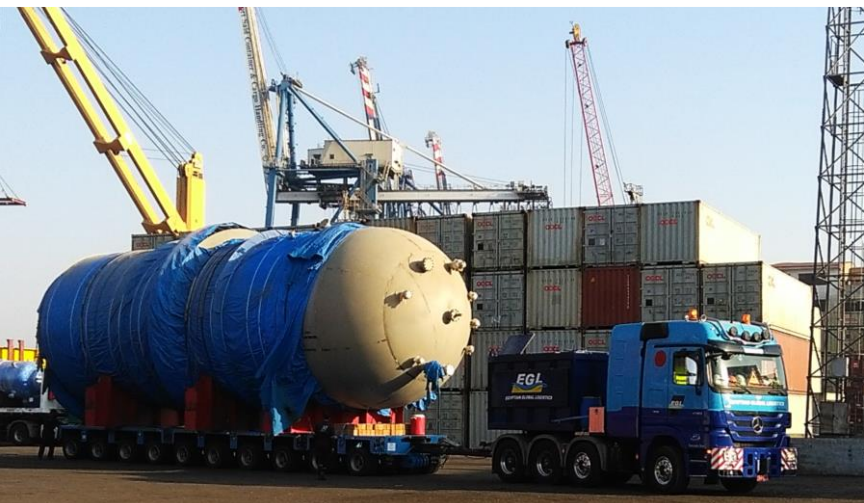
Trucking of Blow Down vessel unit of 72 tons, 17m Long & 6.4 Height from Alexandria to Sokhna
