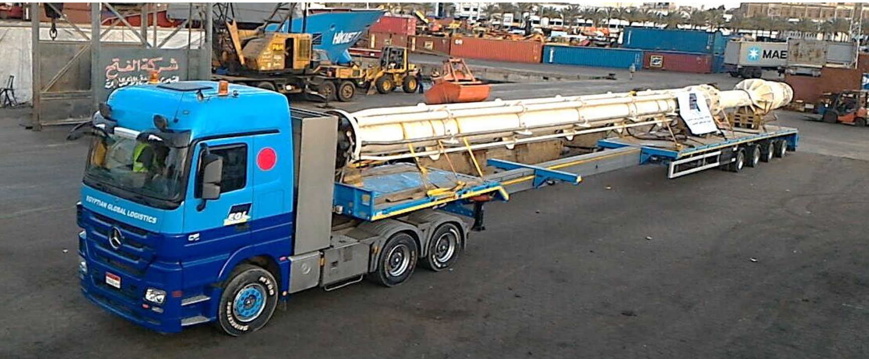
Mediterranean Sea Biggest Gas Discovery, Transport of a Joint of 28 meters long & 40-Tons
