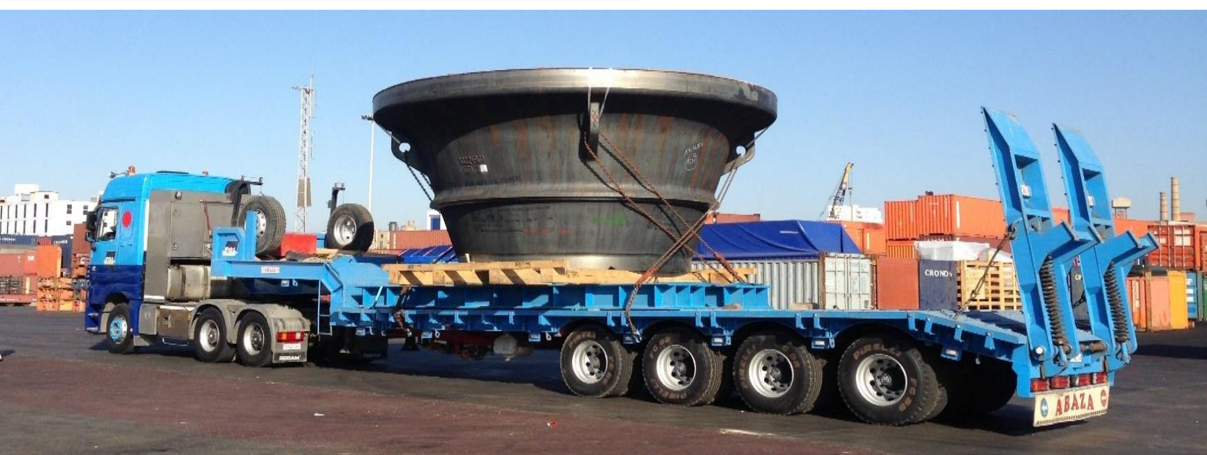
Discharging and Transport of 6 Grinding Tables 60-tons each for cement factory
