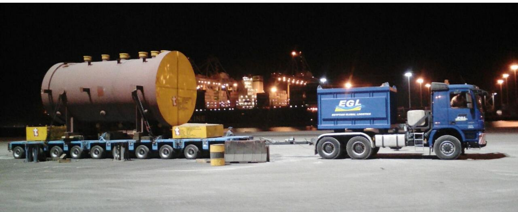
Loading & Trucking boiler of 110 ton from Adabiya port to Sokhna
