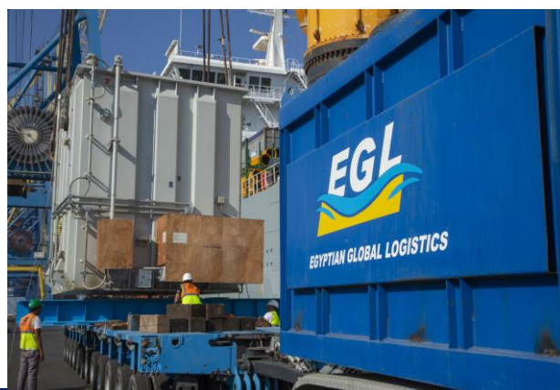
Offloading and delivering 8 transformers each of 228Ton to the yard in Dekhila port
