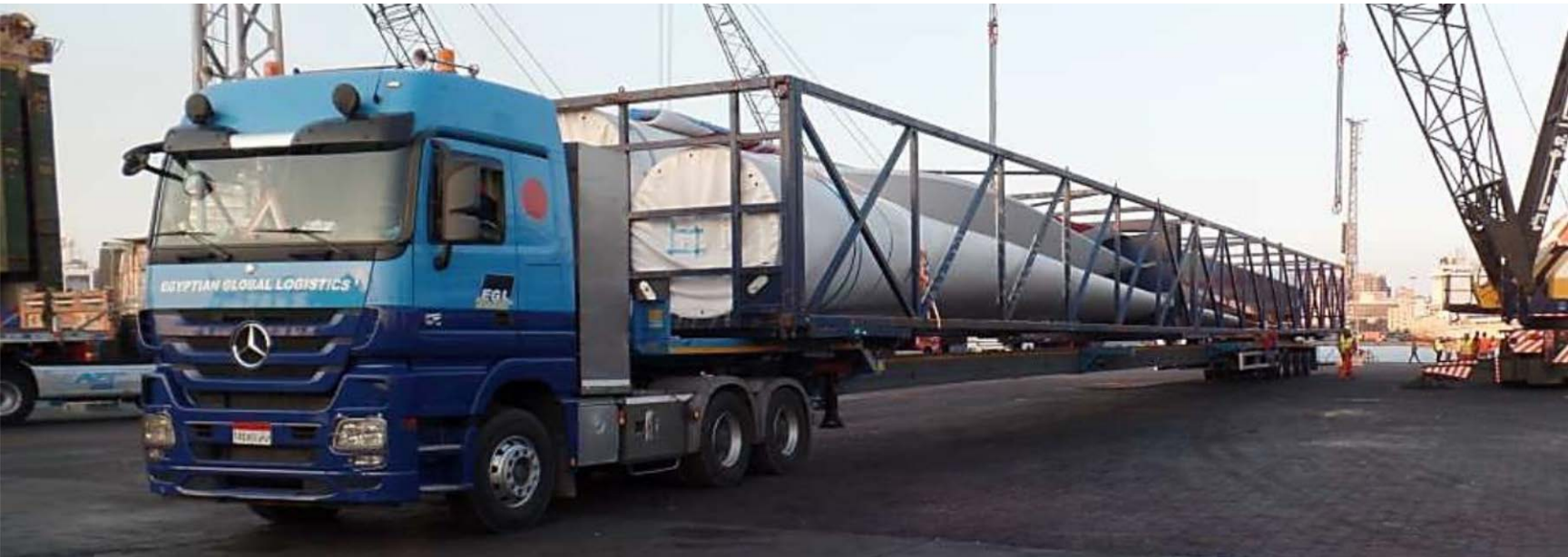
Storage & Transport of Gamesa Blades 49m—28 tons (Extendable) & Nacelle 79-tons (Low bed)
