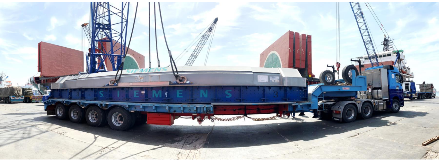
Discharging & Transportation of 72 tons rotor for Siemens in Alexandria port.
