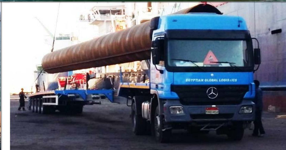
Discharging using floating cranes, Barging & transport of 47 tons 43 m steel pipes to the site at Port Said east new jetty.
