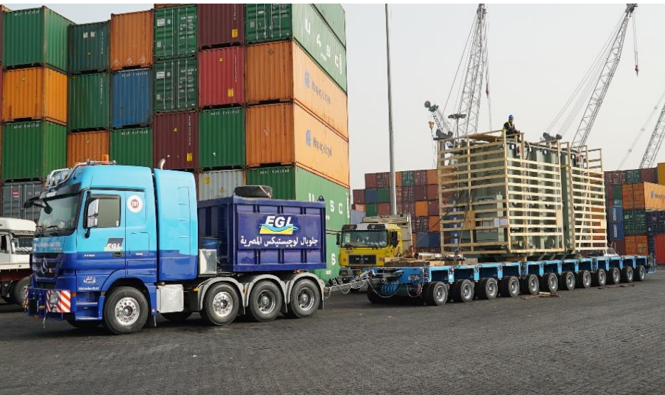
Discharging, Trucking & Unloading to foundation for 2 Siemens Transformers of 135 tons each from Alexandria port to El Galala City.
