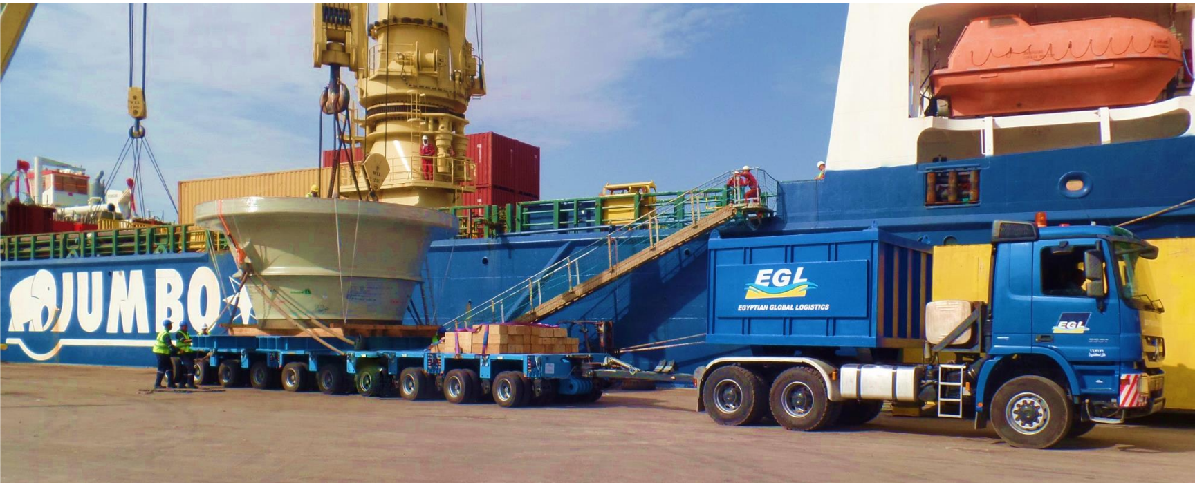
Trucking, Discharging & Storage on Steel Beams & Transport of 3 Grinding Tables 126-tons each from Adabiya port to Beni Suef
