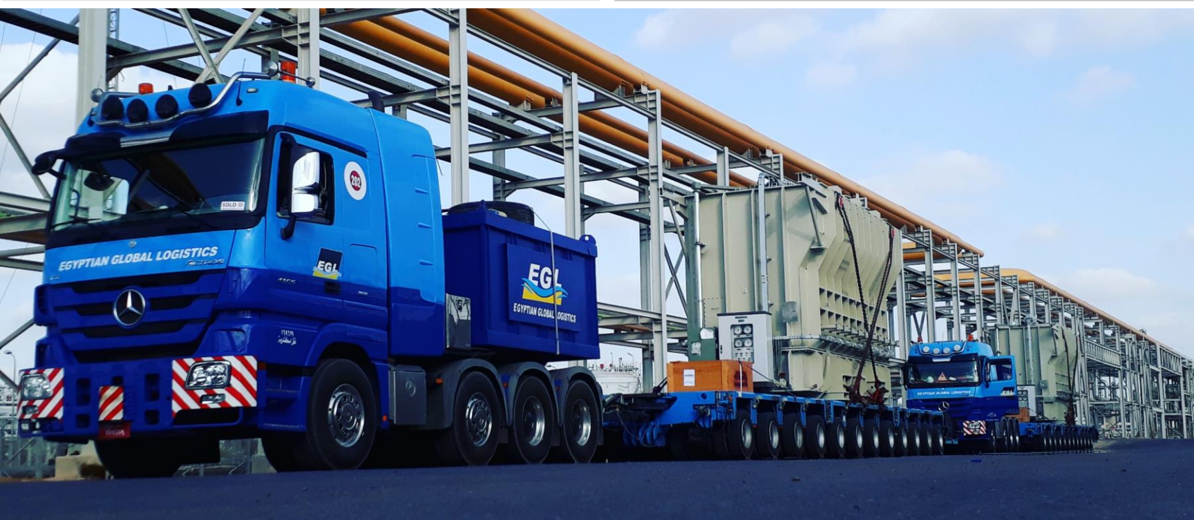
Trucking & Unloading of 2 Transformers of 124 tons each from Cairo to El Nahda Alexandria.
